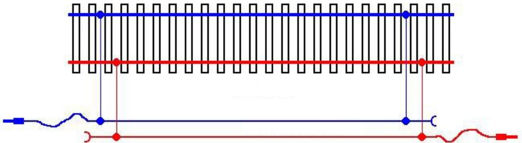
**A DCC Data Bus Cable**, Male-Male, the length of each module plus 18" will accompany each module. At the minimum, one F-F Coupler shall be carried for connecting to other modules. DCC cables can be made to differing lengths using RJ12 connectors and flat 6-wire cable. See "DCC Universal Bus Construction and Components" for more details.
