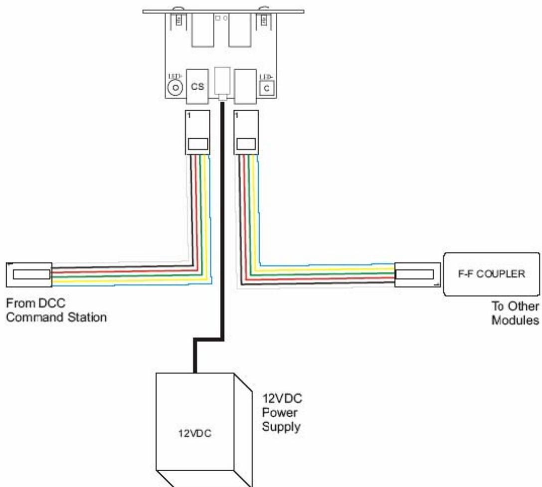
In situations where there are branching modules, the DCC bus should branch as well. This illustrates how a two-way splitter plug can be used to accomplish this branching. Notice that power insertion is indicated on the branch. This may or may not be necessary, depending on system type and the length of the branch.
